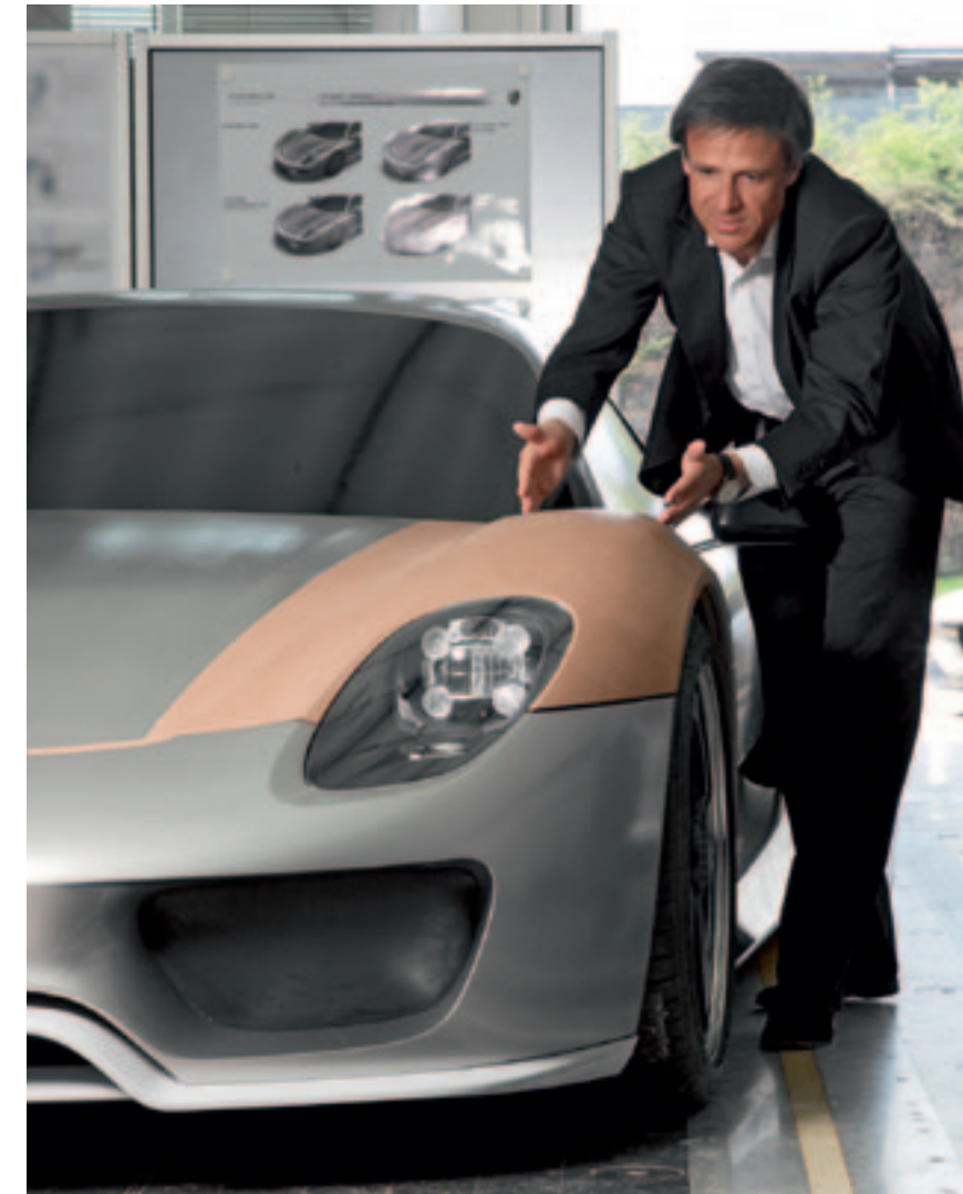
New proportions become tangible on the clay model Am Clay-Modell werden neue Proportionen greifbar
